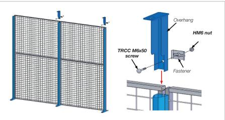
If the wall is higher than the sliding door, install the overhang horizontally in order to fix the rail.
