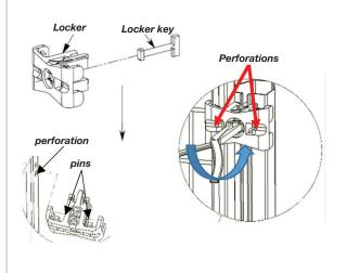
Use 4 lockers for heights 1750/2000/2200/2400. Use 6 lockers for heights 2500/2700/3000. That is to say 2 lockers per panel.
